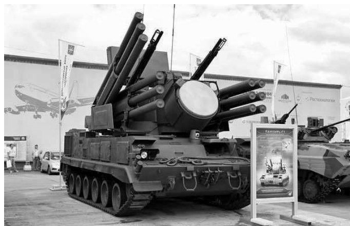
Pantsir-S1 mounted on a tracked GM-352 chassis.
